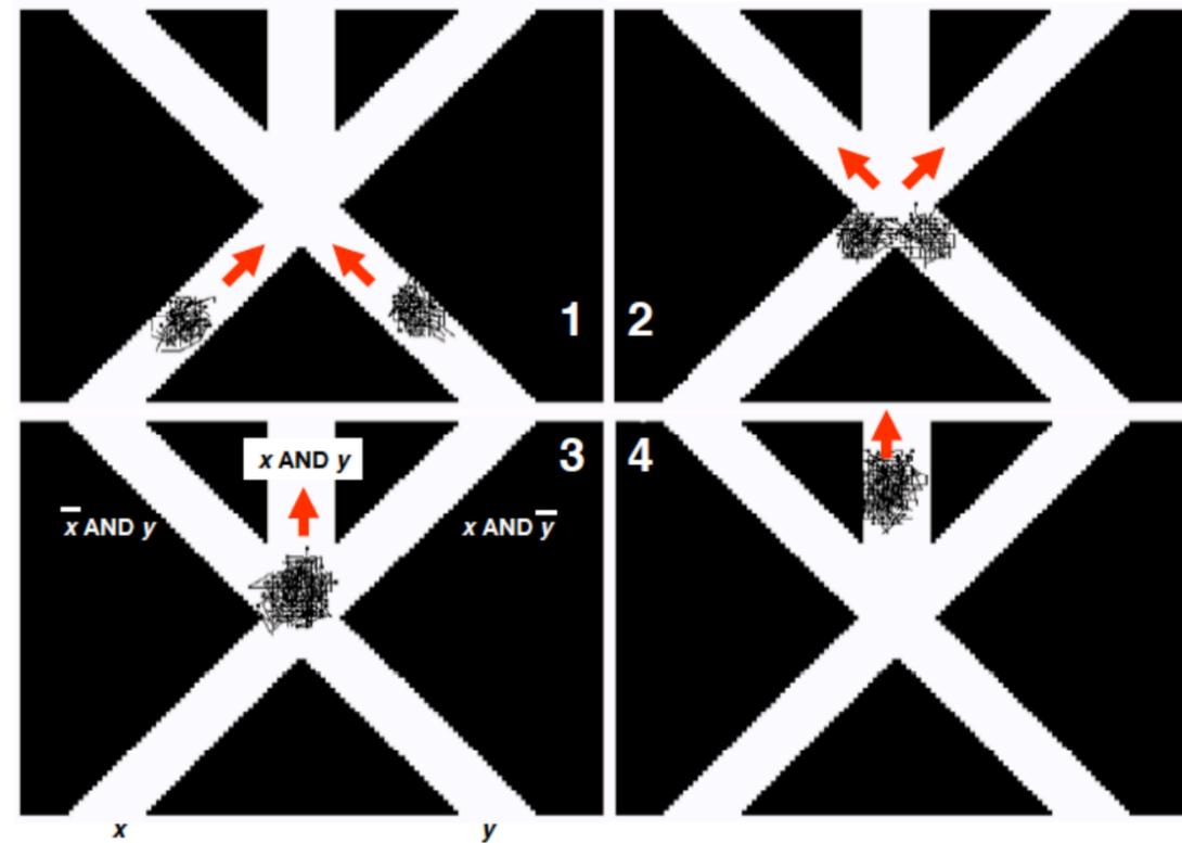
FIGURE 3. A series of snap shots (1, 2, 3 and 4) in AND gate of swarm balls. A swarm ball locate at  $x$ - and  $y$ -position consists of 40 agents, respectively. Each agent is represented by a square with its 5-steps-trajectories. Red arrows represent the direction of motion of a swarm ball.
